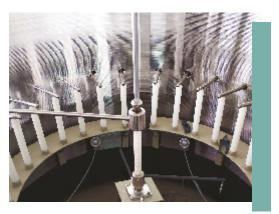
The automated system for research and development testing of high-voltage insulation materials enables accelerated aging of insulation samples, control of humidity, temperature, and independent control of voltage testing. Such a complex testing system enables the market competitiveness of some products of the Končar Group.
