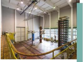
A test of the transformer conductor by heating with a current of 25 kA was performed in the Laboratory Center, for the customer from Sweden. The innovative test method was developed independently and significantly expands the existing possibilities of testing with heating current max. 10 kA.
